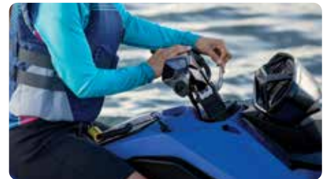
Handlebar With Adjustable Riser A telescopic steering system that optimizes the experience for varying rider sizes.
